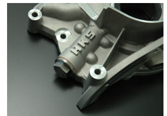
Oil pressure adjustment portion
